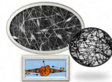
Figure 1: Natural model: Spider web capturing silk with water collection capability. Technical model: Electrospun spindle-knotted structured fibers with underwater micron-oil droplets collection capability.
