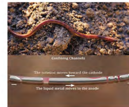
Figure 1: The electric actuation of liquid metal column was similar to the movement of bionic earthworm.
